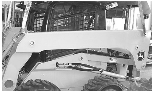
Boom With Hoist And Lifting Straps
