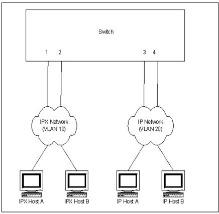
On this switch, the administrator configures all IPX traffic to be bound to VLAN 10. All IP and ARP traffic is bound to VLAN 20. By adding ports 1 and 2 to VLAN 10, and adding ports 3 and 4 to VLAN 20, the administrator ensures that no IPX traffic will be admitted to the IP network. Conversely, no IP or ARP traffic is admitted to the IPX network.
