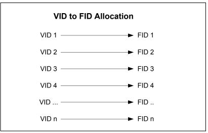
**2.** Ensuring that each FID supported by the bridge is allocated to exactly one spanning tree instance.
