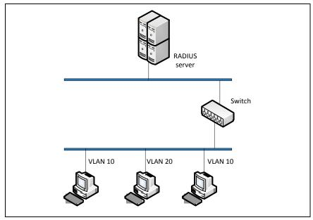
In a standard 802.1X scenario, all subsequent clients in the network that are connected to the same port need not authenticate to use the port on the switch. When MAC-based 802.1X authentication is enabled, all the subsequent clients in the network that are connected to the same port must authenticate themselves to use the port on the switch.
