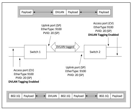
**Uplink port (service provider port):** If a packet ingresses on an uplink port and the packet is tagged only with the service-provider-tag (*SP-tagged*), or the packet is double-tagged (where the SP tag is the outer tag), the switch lets it pass through unchanged to the respective access or uplink ports.
