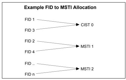
The combination of VID to FID and then FID to MSTI allocation defines a mapping of VIDs to spanning tree instances, represented by the MST Configuration Table. The following figure shows an example configuration:
