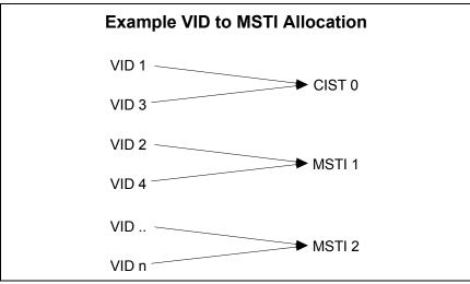
This allocation ensures that every VLAN is assigned to one and only one MSTI. The CIST is also an instance of spanning tree with a MSTID of 0.
