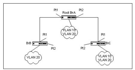
For VLAN 10, this single STP topology presents no limitations or inefficiencies. On the other hand, VLAN 20's traffic pattern is inefficient. All frames from bridge BrB will have to traverse a path through bridge BrA before arriving at bridge BrC. If the ports Pt2 on bridge BrB and BrC could be used, these inefficiencies could be eliminated. MSTP does just that, by allowing the configuration of MSTIs based upon a VLAN or groups of VLANs.
