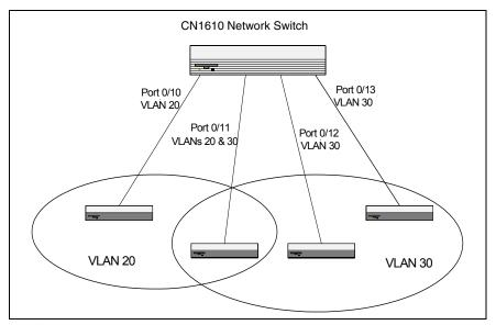
The following examples show how to create VLANs, assign ports to the VLANs, and assign a VLAN as the default VLAN to a port.
