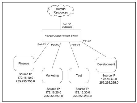
First, DiffServ is enabled. Then, for each department, a class map is configured that matches a source IP address:
